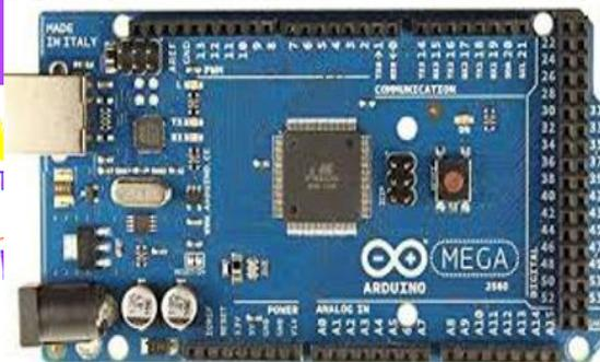
Gambar 2. Arduino Mega2560.
